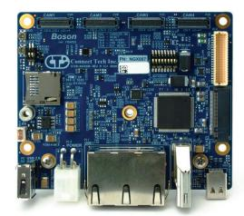
Equipped with 4x FRAMOS PixelMate connectors for instant access to the entire FRAMOS Sensor Module Ecosystem.
