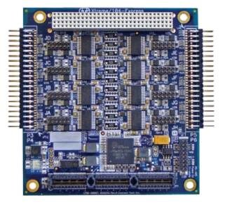
Xtreme/104-Express is Connect Tech's first PCI/104-Express multi-port serial board. Fully PCI/104-Express compliant, this board provides a PCI-104 pass-through connector for easy transition from legacy PCI-104 cards to PCI Express stacks.
