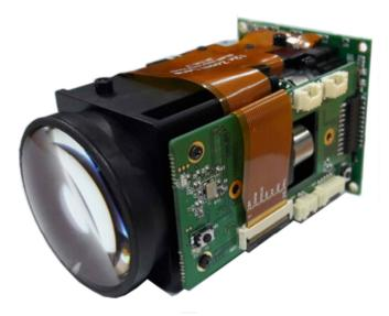
*EEM012-HDSDI* is an BT1120 output format vision camera . With its compact design. *Key Features*
